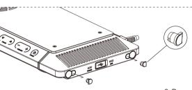
Remove the the rubber stoppers on both sides of the light.
