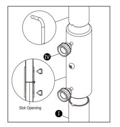
Insert Arm and Extension Tube (I) into Coupling (II) until they meet the slot opening. Use two M5 Thumb screws (IV) to secure both tubes.
