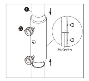
Insert both Extension Tubes (I) into Coupling (II) until they meet the slot opening. Use two M5 screws (IV) to secure both tubes.
