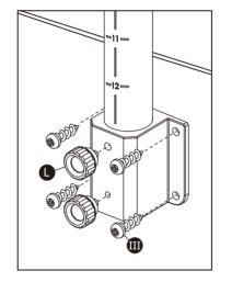
Use four M4 Phillips Wood screws (III) to secure the Tube Adapter on wood stand. Put Extension Tube (I) into the Tube Adapter. Secure them with two M5 Thumb screws.
