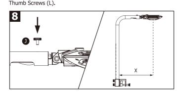
Adjust the position of the Slide Bar according to your aquarium width. Secure with M3 Thumb Screw (J). Length X should be half of your aquarium width. For 18" width, X=9"; For 24" width, X=12".
