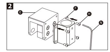
Insert four M4 Round Head Hex screws (H) through Tube Adapter (F) and into Arm Mount (E). Secure with M4 Hex Key (N).
