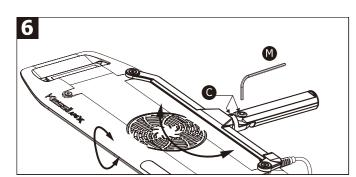
After adjusting the angle of the AP9X Bracket + Slide Bar (A), tighten and secure the M6 Cap Head Hex Screw (C) with M6 Hex Key (M).
