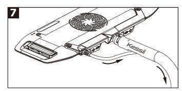
Fit the AP9X power cord through the slot on the Arm (D) and all the way to the bottom. Slide the AP9X and AP9X Bracket + Slide Bar (A) into Arm (D).
