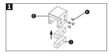
Insert two Steppers (I) into the Arm Mount (E) and secure them with four M5 Phillips Cap screws (K), using a Phillips screwdriver.
