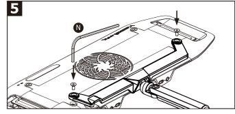
Use M4 Hex Key (N) to secure the AP9X Bracket + Slide Bar (A) and AP9X together with the two M4 hex socket cap screws from Step 4.
