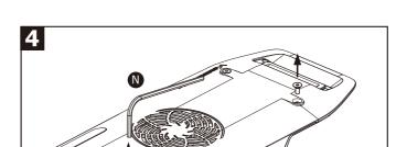
Remove the back two screws from the top side of AP9X, using M4 Hex Key (N). Keep these two screws for the next step.
